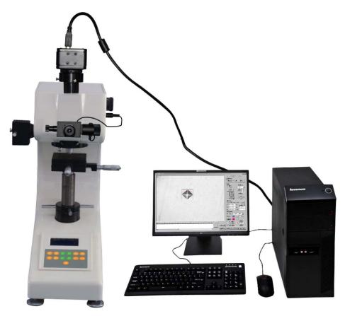
This machine is equipped with a micro hardness tester system: it can be used for continuous test of continuous indentation after continuous loading, and can carry out successive experiments for each load and each indentation. Using a digital camera with a convenient ccd camera, video cable, or USB interface, the measurement indentation can be directly observed on the monitor, and the accuracy can be measured with the mouse.
